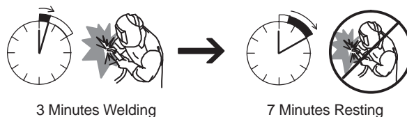
30% Duty Cycle At 210 Amperes
