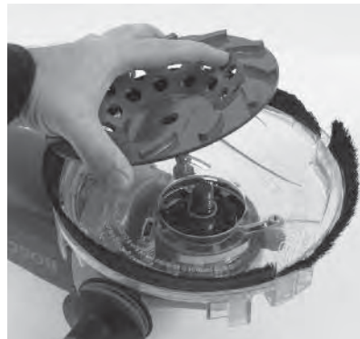
4. Install grinding wheel. (Use the washers provided to adjust wheel slightly below the brushes. You may also adjust the 3 screws if needed)
