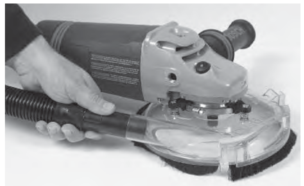
5. Insert hose to port. Secure other end of hose to the electric cord with releasable tie provided.
