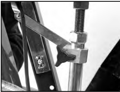
(A) Lubricate the Depth Control Screw (Monthly).
