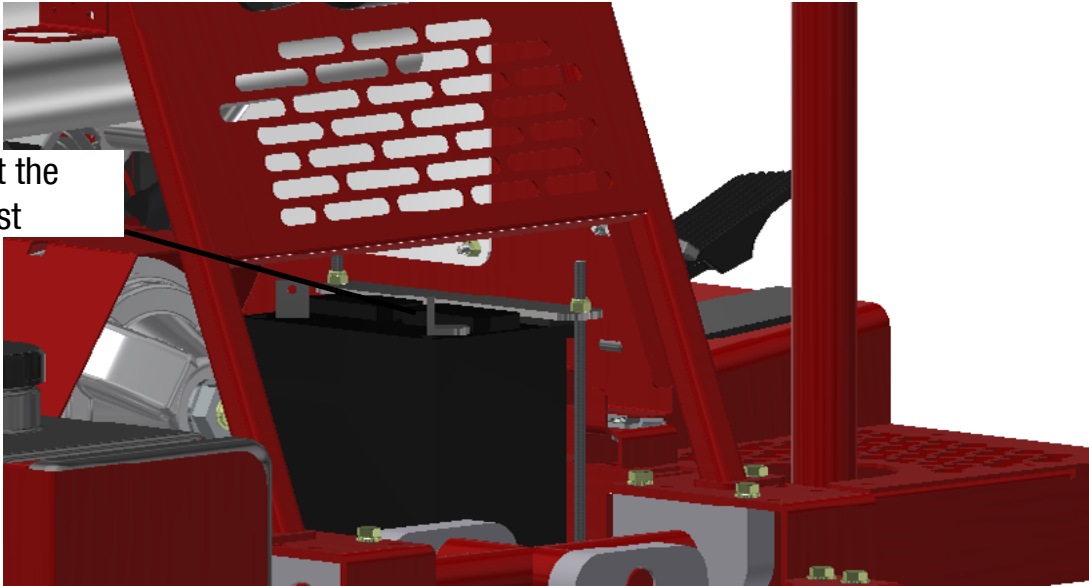
Figure 3.2: Battery and Plate
