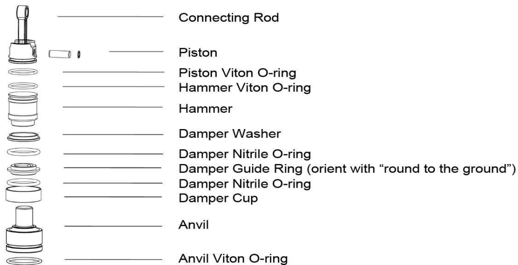
Figure 9: View of the orientation of internal parts
