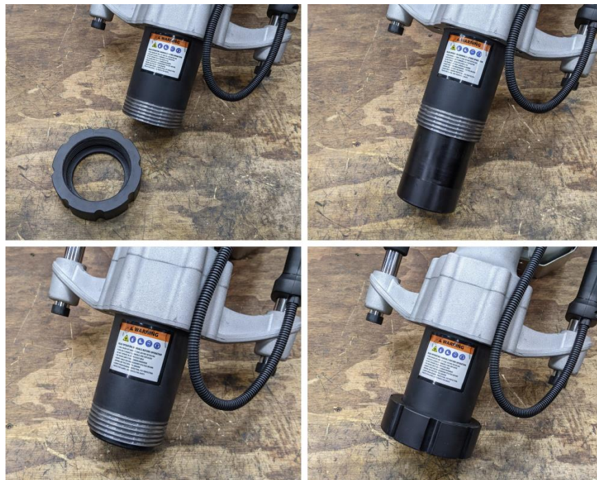
Figure 2: Installing the adapter sleeve on a PGD3200X
