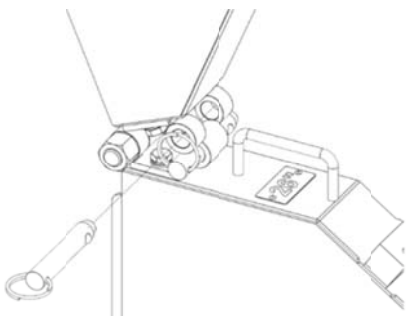
Figure 14: Second Lock Pin through Ring of First
