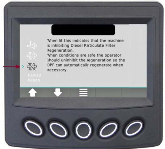
Figure 46: Inhibiting DPF Regeneration Screen
