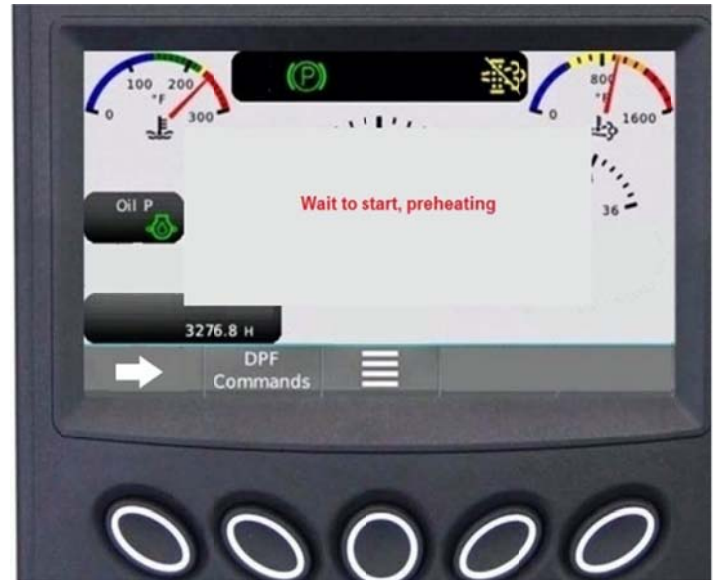
Figure 35: Preheating Warning Message
