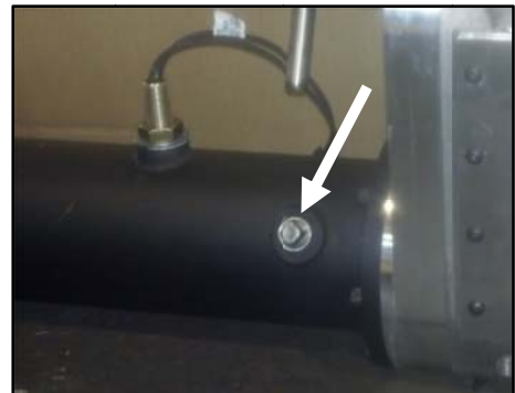
Figure 83: 3/8" Overflow Pipe Plug
