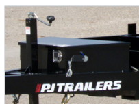
SELF-CONTAINED HYDRAULIC UNIT & FRONT-LOCKING TOOLBOX
