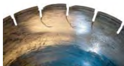
Cracked Segments and/or Core Wrong Blade for the job
