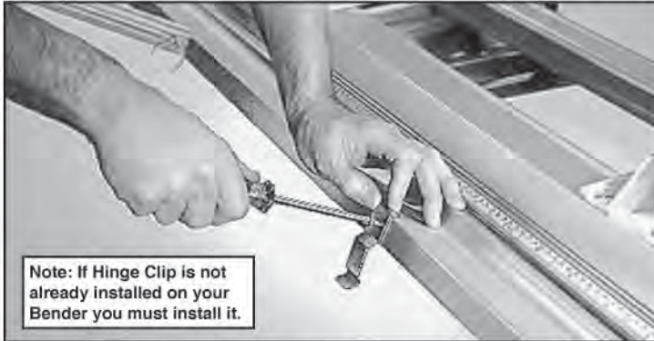
Figure 1. The Hinge Clip keeps the Moving Hinge in a 90° position for ease of aligning and cutting material. To install Hinge Clip, locate pre-drilled hole on BOTTOM right side of Moving Hinge. Align holes in Clip and Hinge as shown and insert Phillips head screw provided.
