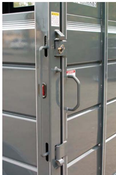
Rear Slam and Latch Design
