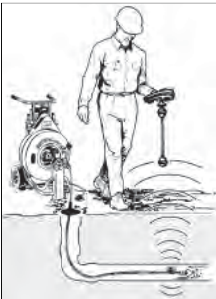
Scout and Remote Transmitter accurately locate problems in the line.
