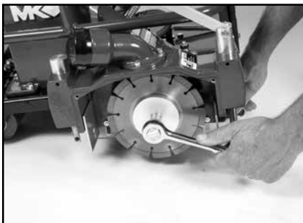
(D) Install the Outer Flange and Blade Shaft Nut. Tighten Blade Shaft Nut holding the Blade Shaft steady.
