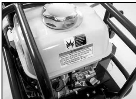
(A) Remove the Fuel Cap. Refer to Engine Manual for details.
