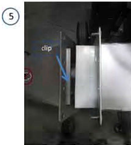
Outlet Tube being re-assembled with clip to support and push liner into final position.
