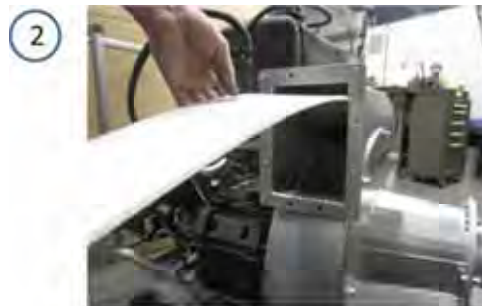
2 Liner pushed against upper section of vacuum housing. The inserted into vacuum.
