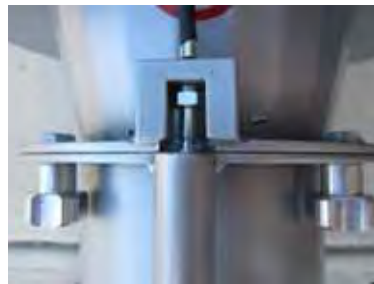
Inlet Safety Switch
