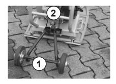
Arrest the guide bar (1) with the spring bolt (2).
