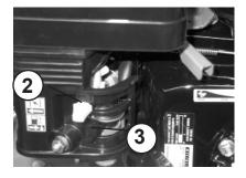
Slowly tighten the handle (1) of the reversing starter (2) until resistance is noticeable.
