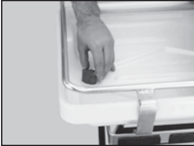
(A) Remove the Drain Plug
