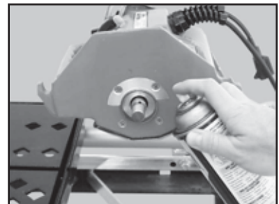
(F) Lubricate the Motor Shaft and Inner Flange
