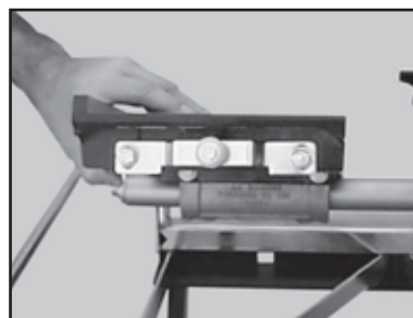
(B) Check the movable Cutting Table Roller Wheel for wear replace if necessary
