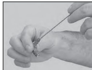
(H) Clean the Blade Guard Intake Fitting, go to Step I.
