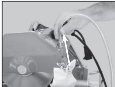
(B) Remove the Transfer Tube from the Blade Guard inlet, go to Step C
