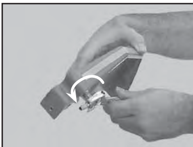
(G) Remove the Blade Guard Intake Fitting, go to Step H.
