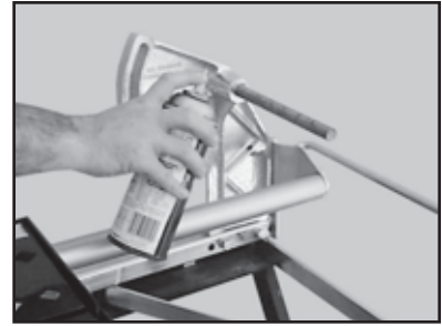
(L) Lubricate the Cutting Head Pivot Shaft
