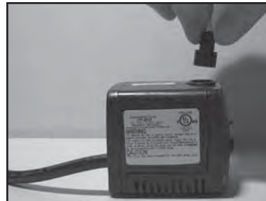
(E) Remove the Pump Discharge Fitting and check flow. If flow exists, go to Step F.
