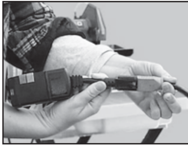
(B) Verify all plugs fully installed
