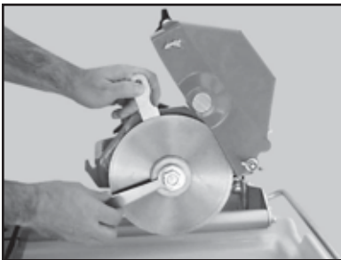
(A) Remove the Diamond Blade
