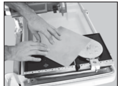
(F) Position the tile against the Protractor and the Ruler/Stop
