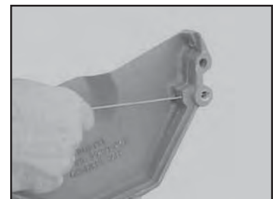
(I) Rod Cooling Channels and recheck flow
