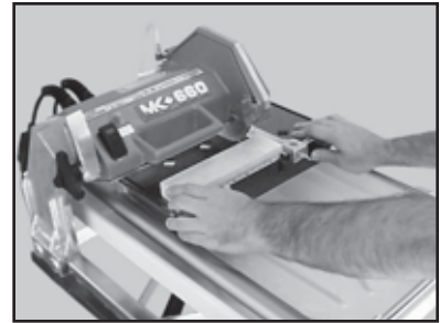
(F) Cut the Dressing Stick seven (7) or eight (8) times to dress the Blade
