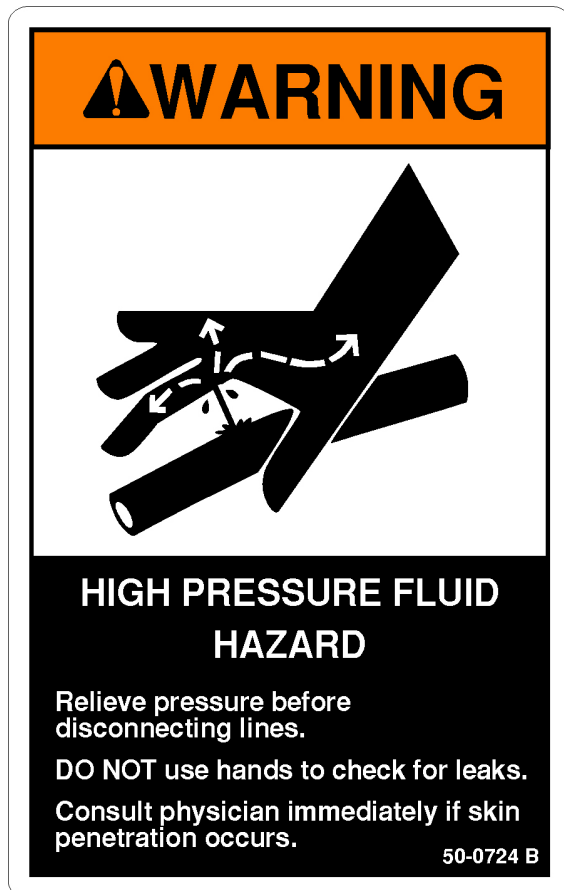
# 50-0724 WARNING! HIGH PRESSURE FLUID HAZARD
