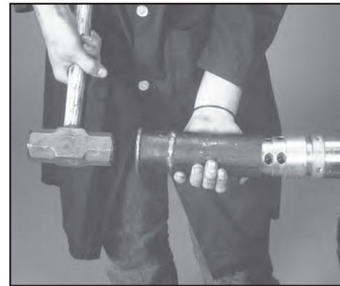
FIG. 31: USING PIPE TO SECURE STEPPED CONE
