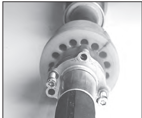
FIG. 58: 2 SCREWS USED AS JACK SCREWS
