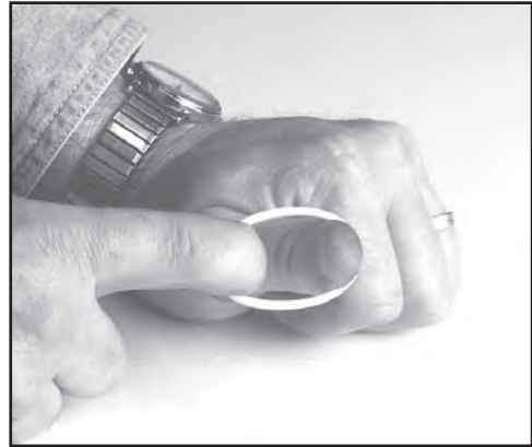
FIG. 46: STRETCH NEW SEAL TO FIT CONTROL STUD
