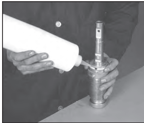
FIG. 30: GREASE THE SEAL
