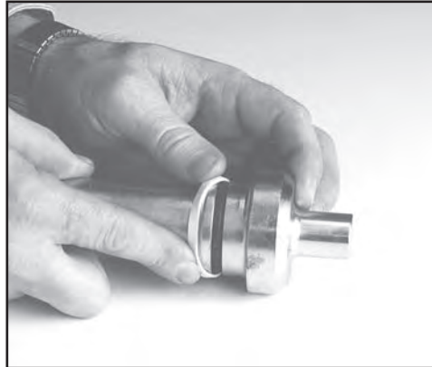
FIG. 25: SLIDE CHISEL SEAL ONTO CHISEL
