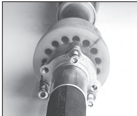
FIG. 57: REMOVE 3 SOCKET HEAD CAP SCREWS
