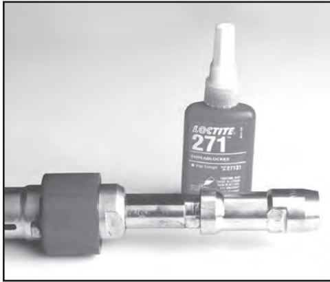
FIG. 51: APPLY LOCTITE AND TIGHTEN CONTROL STUD ADAPTER
