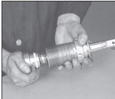
FIG. 27: INSERT THE CHISEL
