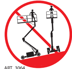
ART_3064 DO NOT ELEVATE OR DRIVE ELEVATED ON A SURFACE THAT EXCEEDS THE LEVELING RANGE
