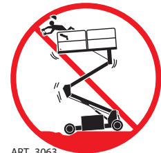
ART_3063 DO NOT DRIVE ON IRREGULAR OR UNSTABLE SURFACE
