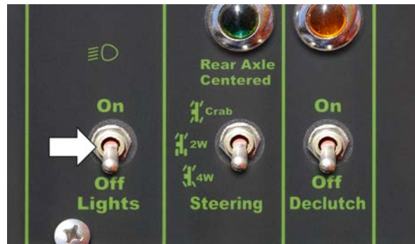
Figure 6-28. Work Light Switch.
