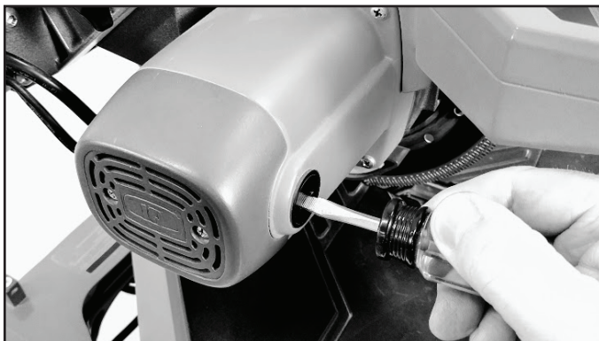
Remove carbon brush retainer cap.
