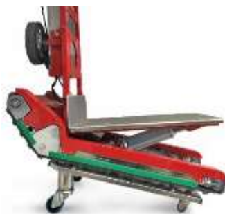
Fig. 88: The tracks of the Domino Automatic trolley are positioned above the "narrow landing base" accessory.
