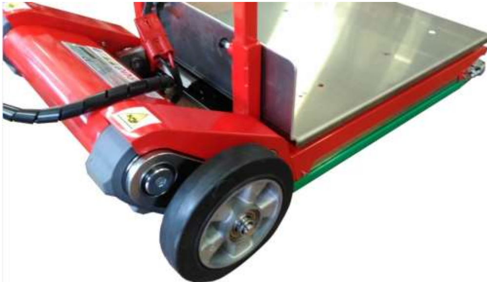
Fig. 59 Wheels correctly fitted on the stair climbing trolley
