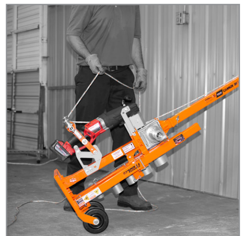
Built-in rope engagement capstan switch
