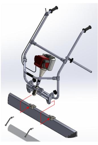
Tools are not required for the assembly of your Multivibe Vibrating screed.
