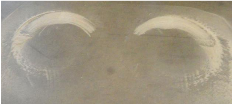
If you see partial circles repeat the process until complete circles are achieved.
