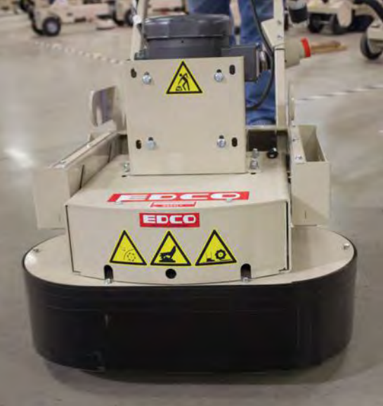
Lean back slightly on the handle to get the tools off the surface and start the machine. Lower the machine to the surface and do a short touch pass on the concrete.
