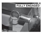
8. Storing the Forks Using two hands, pull out on the two spring-loaded rings located above the fork arms. Slide the fork assembly up off of the carriage while pulling out the rings. The fork can be placed behind the lift for storage.
