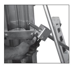
7. Folding the Base Legs Lower the carriage all the way down and engage the Mast Hold Down Bar.
