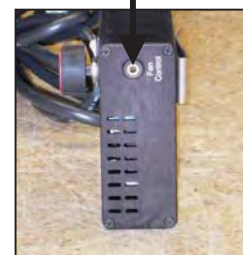
Fan control jacks.
