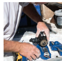
3. Place new pump into sprayer.
