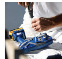
1. Remove the cover with a screw driver.
