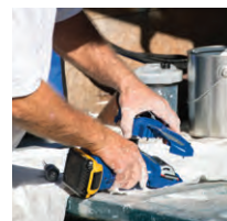
2. Remove the old pump from the sprayer.
