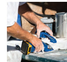
2. Remove the old pump from the sprayer.
