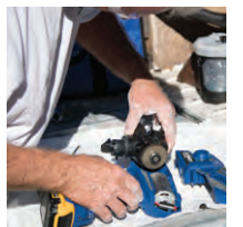
3. Place new pump into sprayer.
