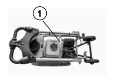
Fit the crane hook into the lifting ring (1) and lift the machine onto the desired means of transport.
