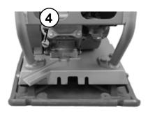
The correct oil level is between the min. and max. marks.
