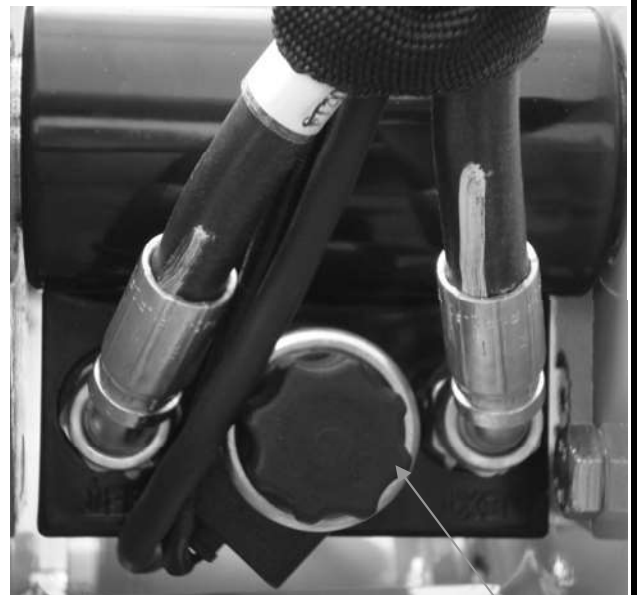
Figure 5-7. Cylinder Valve Removal
