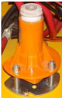
Figure 4-11. Level Sensor Pendulum Based
