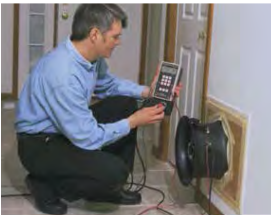
The fan can mount directly to the HVAC system when pressuring the ductwork.
