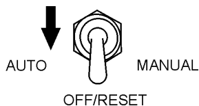
Figure 48. Auto Off/Reset Manual Switch (Off/Reset)
