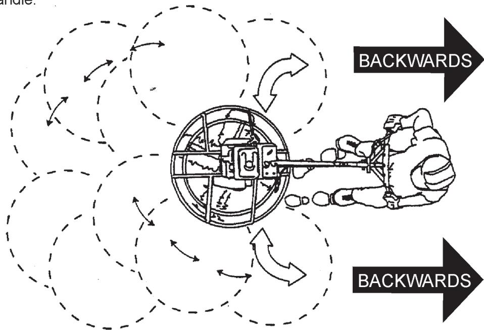
The best method for finishing concrete is to slowly walk **backwards** with the trowel, guiding the trowel from side to side. This will cover all footprints on wet concrete.
