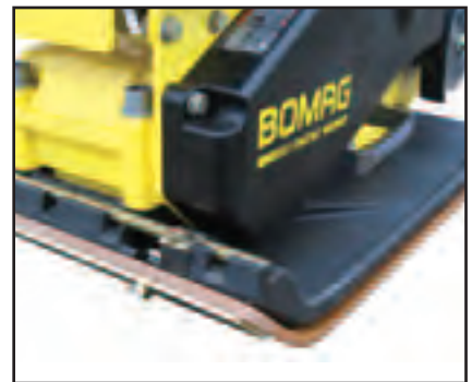
The Vulcolan mat helps to avoid damage to paving stones surfaces.
