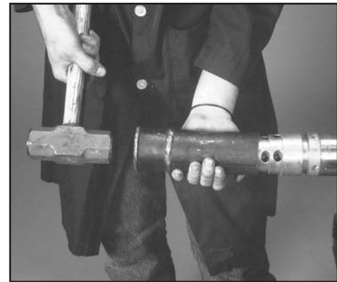
FIG. 31: USING PIPE TO SECURE STEPPED CONE
