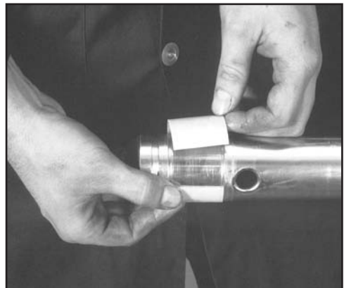
FIG. 73: POSITION REAR SLIDE TAPE
