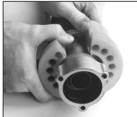
FIG. 69: PLACING ELASTIC BLOCK ON CONTROL TUBE
