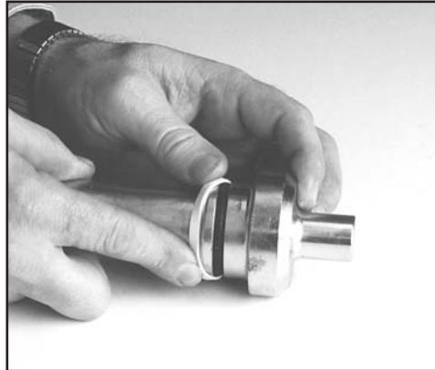
FIG. 25: SLIDE CHISEL SEAL ONTO CHISEL
