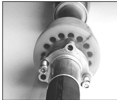
FIG. 54: 2 SCREWS USED AS JACK SCREWS
