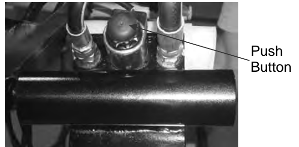
Figure 5-3. Location of Manual Lowering Valves for Lift Cylinder Replacement
