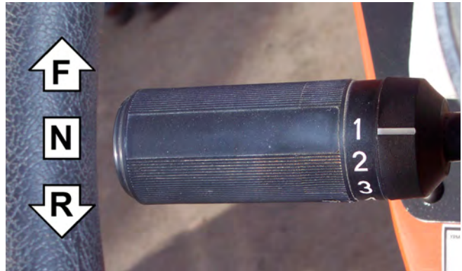
Figure 7-7. Travel Select Lever Must Be In NEUTRAL (N) To Start The Reach Forklift.
