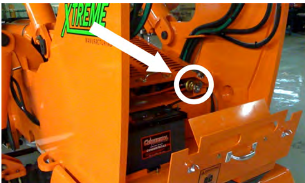
Figure 8-5. Battery Disconnect Switch.
