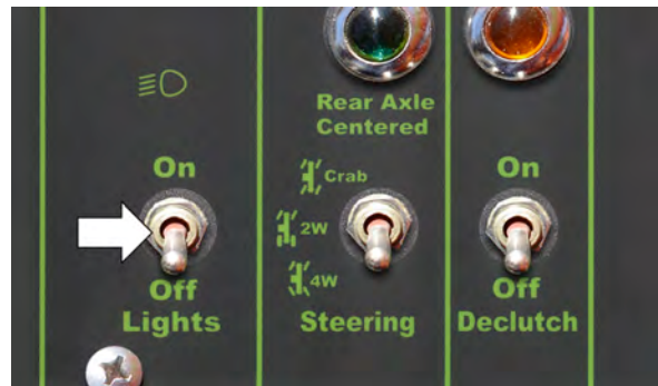
Figure 6-28. Work light Switch.
