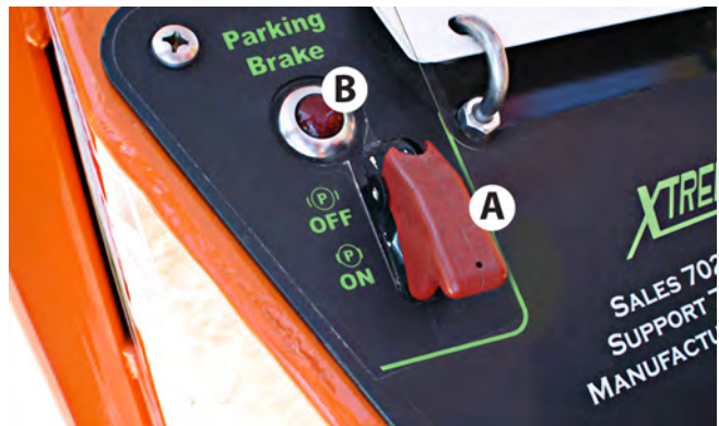
Figure 7-8. Parking Brake Switch (A) Must Be ON (Engaged) To Start The Reach Forklift.
