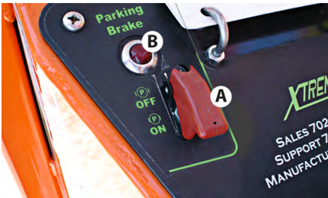
Figure 6-18. Parking Brake. (A) Parking Brake Switch Guard. (B) Parking Brake Indicator.
