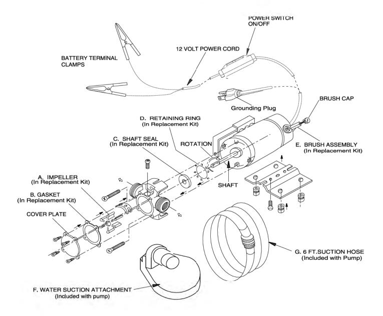
Figure 3 - Replacement Parts Illustration for Self-Priming Transfer Pumps
