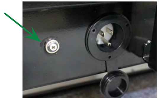
The reset button is located next to the charging port on the Ride On Carts.
