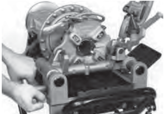
Figure 10 – Threading Pipe With No. 811-A Quick Opening Die Head
