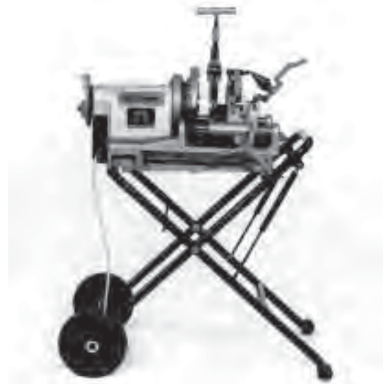
Figure 2 – 300 Compact on 250 Folding Wheel Stand
