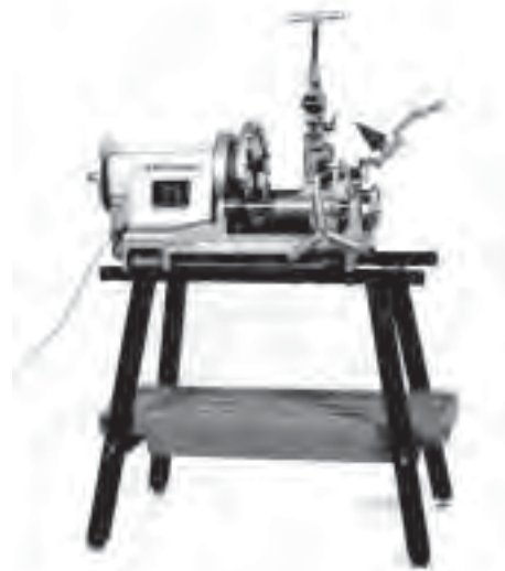
Figure 5 – 300 Compact On 100A Leg and Tray Stand
