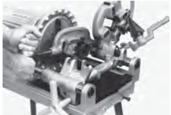
Figure 7 – Cutting Pipe With 300 Compact Threading Machine
