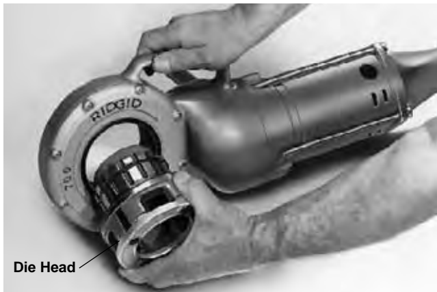
Figure 3 – Installing No. 12-R Drop Head Die Head
