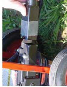
2 Snap torque tube onto connector at engine end.
