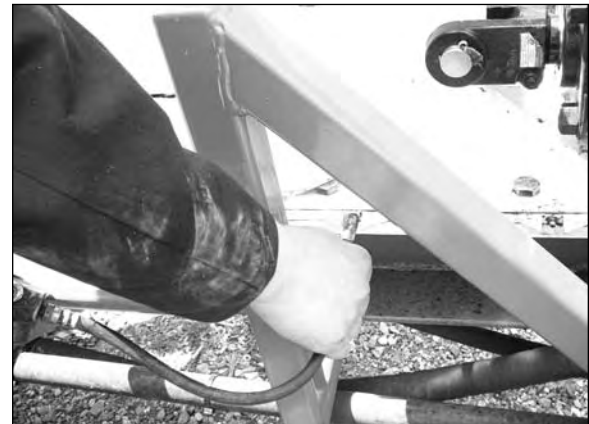
Step 3 With the splitting wedge in the forward position lubricate the slide rails with high quality grease. This will help to prevent wear between the slide plates and the slide rail.
