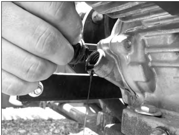
Step 2 The engine’s crank case must be filled with the engine manufacturer’s recommended oil.
