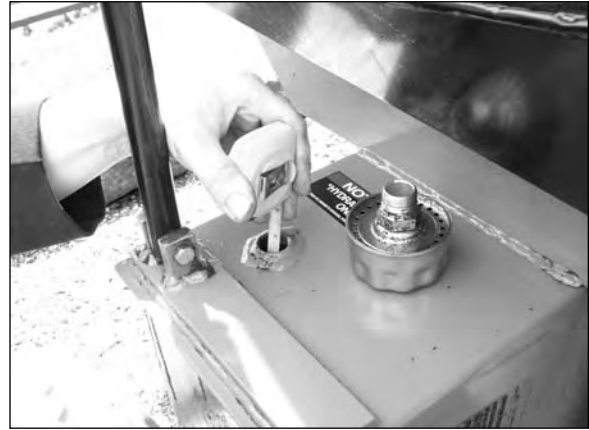
Step 1 Remove cap to check to ensure that there is sufficient hydraulic fluid in the reserve tank. Fluid level should be approximately two inches from the top of the tank. If necessary add only SAW46 high quality hydraulic fluid. NOTE: The total hydraulic system oil capacity is 80 quarts.
