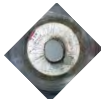
Arbor Hole Out-Of-Round Blade not properly tightened or seated on arbor.
