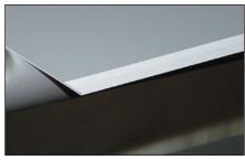
D. Standard Hem. Hems can be formed on all Mark Series<sup>™</sup> brakes, TrimMaster<sup>®</sup> brakes and Metal Master<sup>®</sup> 20 brakes. Visit www. van-mark.com for more tips and ideas.
