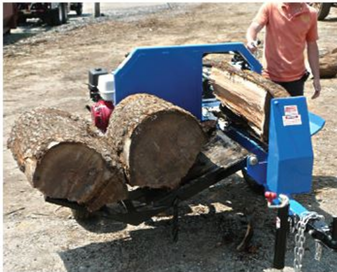
Mighty Ox Log Lifter is rated to handle 1,200 pounds. It also serves as a handy work station for lining up multiple logs for splitting.
