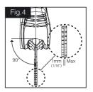
If the gap between the blades is too large, remove and gently bent inward to adjust the gap. Ensure that both blades are aligned vertically to the tool (See fig.4).
