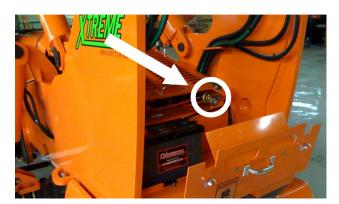
Figure 8-5. Battery Disconnect Switch.
