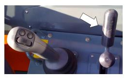
Figure 7-34. Frame Sway Control Handle.
