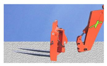
Figure 7-21. Position Quick Attach Adapter In Line With Attachment.
