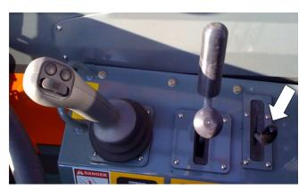
Figure 7-19. Auxiliary Attachment Control Lever.
