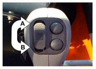
Figure 6-39. Attachment Tilt Switch.
