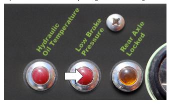
Figure 6-21. Low Brake Pressure Indicator.
