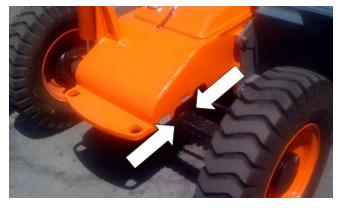
Figure 2-1. Brake Release Bolts.
