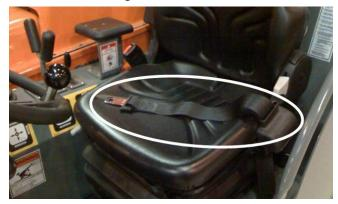
Figure 6-13. Retractable Seat Belt.
