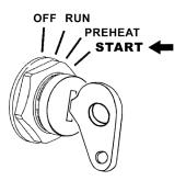
Figure 7-11. Turn Key In Ignition Switch To START.
