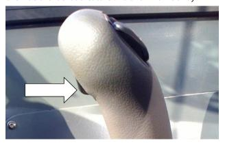
Figure 7-36. Frame Sway Override Switch.
