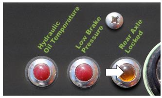
Figure 7-16. Rear Axle Lock Indicator.
