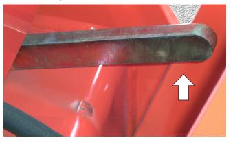
Figure 7-30. Raise Quick Attach Lock Lever.
