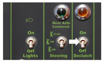
Figure 6-33. Declutch Switch.
