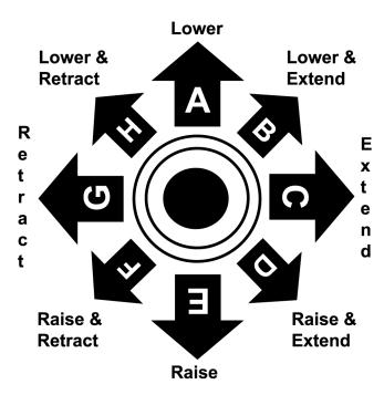
Figure 6-38. Boom Control Handle Functions.
