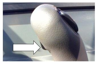
Figure 6-41. Frame Sway Override Switch.
