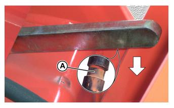
Figure 7-27. Make Sure Quick Attach Lock Lever Is Seated In Groove (A) of Quick Attach Pin.
