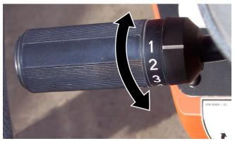
Figure 6-17. Gear Select Switch.
