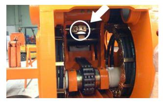
Figure 8-3. Extend Cylinder Lower Down Valve.
