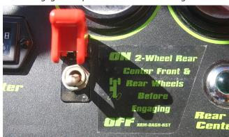
Figure 6-43. Two Wheel Rear (2WR) Steering Switch.
