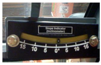
Figure 6-46. Frame Level Indicator.
