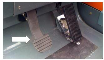
Figure 6-5. Service Brake Pedal.
