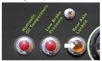
Figure 6-22. Rear Axle Lock Indicator.
