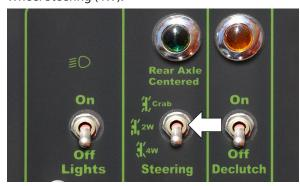
Figure 6-31. Steering Select Switch.
