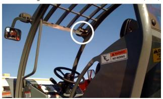
Figure 7-35. Frame Level Indicator.
