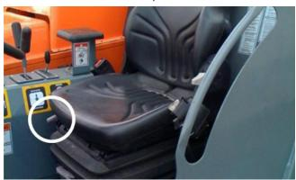
Figure 6-11. Fore and Aft Adjustment Lever.
