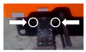
Figure 2-2. Brake Release Bolts (Cab Side).
