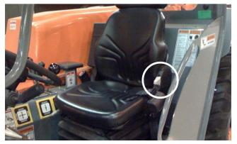
Figure 6-12. Backrest Angle Adjustment Lever.
