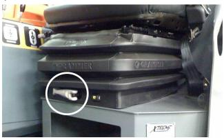
Figure 6-9. Weight Suspension Lever.
