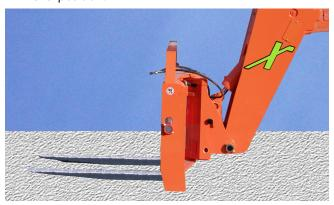
Figure 7-32. Lower Attachment to Ground in Level Position.
