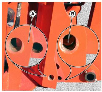
Figure 7-24. Tilt Attachment To Align Holes Between Quick Attach Adapter and Attachment.
