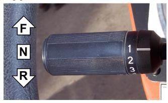
Figure 7-7. Travel Select Lever Must Be In NEUTRAL (N) To Start The Reach Forklift.
