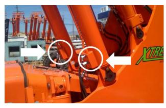
Figure 8-4. Lift Cylinder Lower Down Valve.
