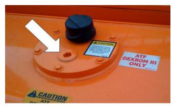
Figure 7-2. Add Hydraulic Oil, If Necessary.
