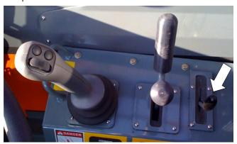
Figure 6-42. Auxiliary Attachment Control Lever.
