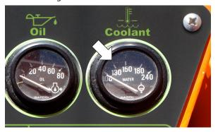
Figure 6-27. Coolant Gauge.
