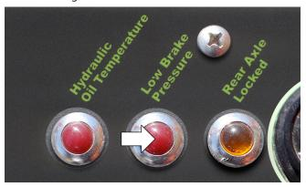
Figure 7-15. Low Brake Pressure Indicator.
