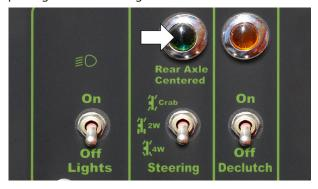
Figure 6-30. Rear Axle Centering Indicator.
