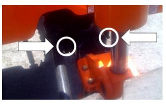
Figure 2-3. Brake Release Bolts (Tank Side).
