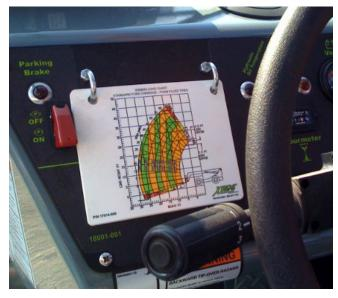
Figure 6-19. Typical Load Capacity Chart.
