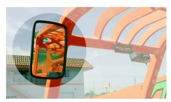
Figure 6-14. Cab-Mounted Mirror.
