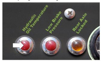
Figure 6-20. Hydraulic Oil Temperature Indicator.
