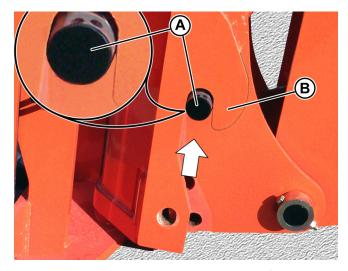
Figure 7-23. Raise Boom To Seat Pivot Pins (A) In Attachment Hooks (B).
