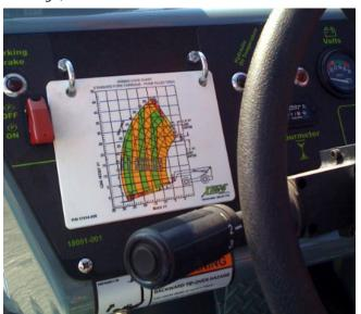
Figure 7-37. Typical Load Capacity Chart.
