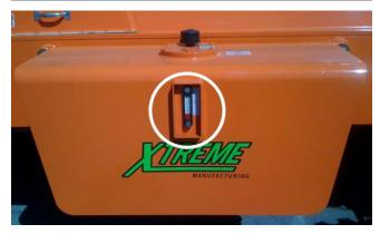
Figure 7-1. Check Hydraulic Oil Sight Gauge.
