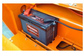
Figure 7-5. Check Battery Case and Terminals.
