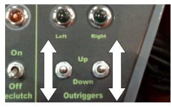
Figure 6-34. Outrigger Toggle Switches.
