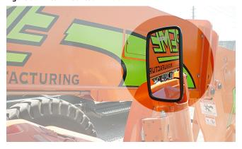
Figure 6-15. Frame Mounted Mirror.
