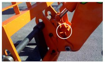
Figure 7-25. Raise Quick Attach Lock Lever.
