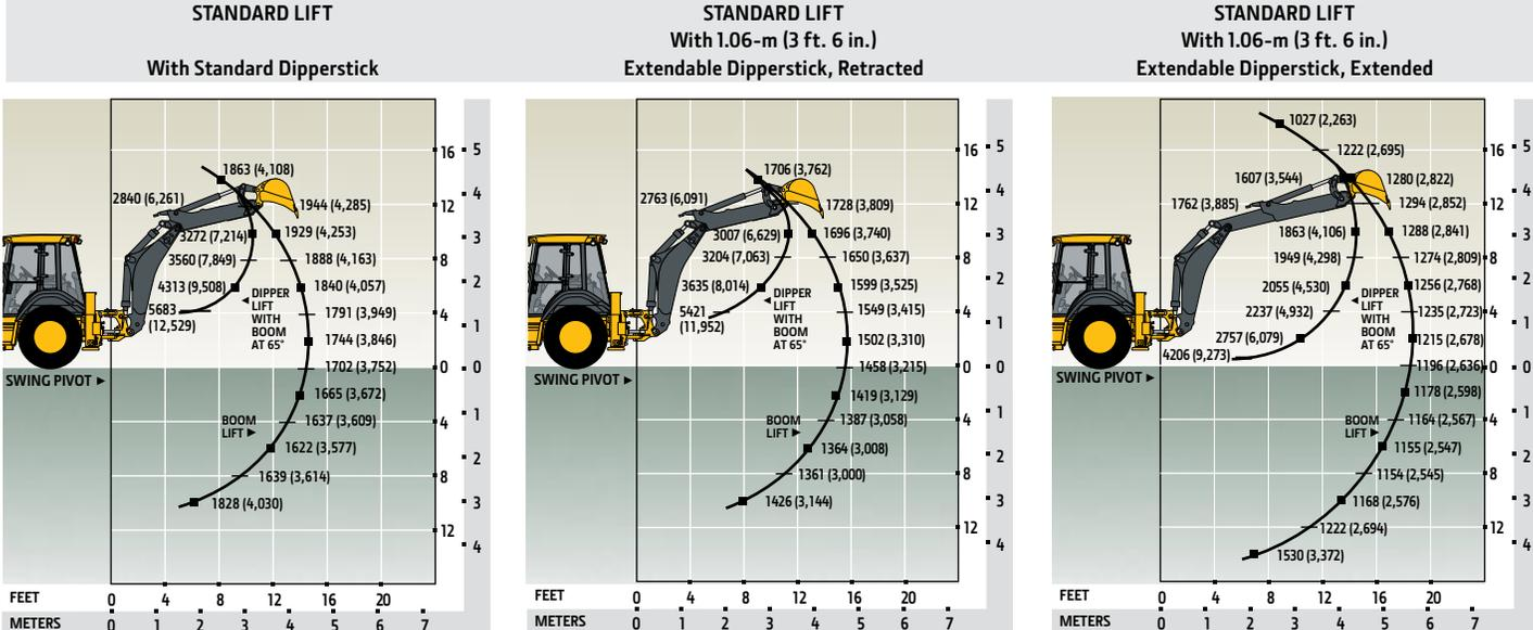
\*Indicates capacity is stability limited. Lift capacities are over end with stabilizers down and tires tangent to ground.
